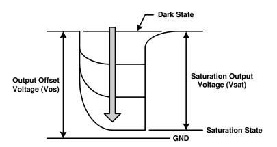
xi Difference between output signal under dark conditions and Vref with an integration time of 1 ms.
